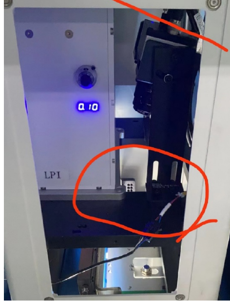
Figure 6-14 Light source not in parallel with the camera
