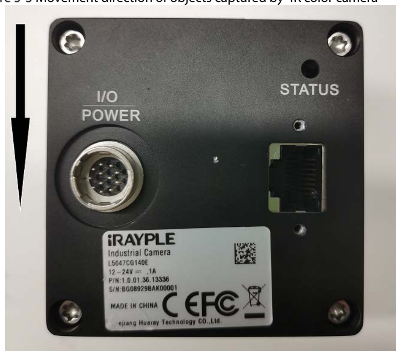
Figure 5-4 Movement direction of objects captured by 8K color camera
